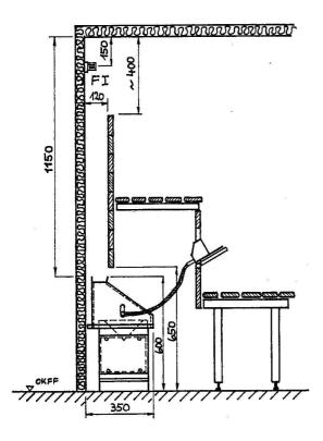
Place the Saunaheater in front of the air intake opening.
